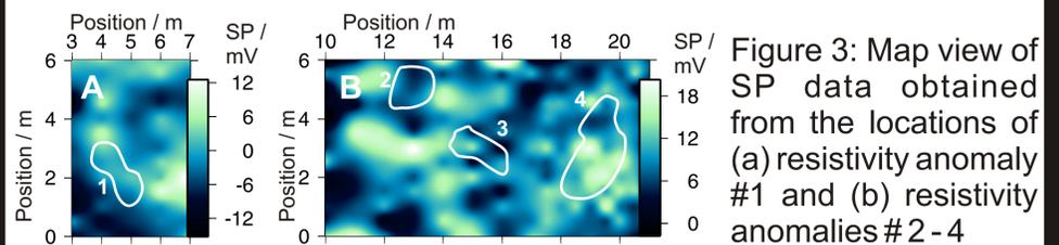
Figure 3: Map view of SP data obtained from the locations of (a) resistivity anomaly #1 and (b) resistivity anomalies #2-4. An area of high SP values (light blue) can be seen in the lower half of anomaly #4 whilst the other three features are comparable to background SP values (Fig. 3). Hence, from this investigation, it is recommended that excavation of the garden begins at anomaly #4, before moving on to features #1, #2 and #3 if nothing is found.
