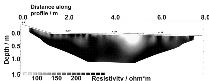
Figure 4: ERT data taken from the crime scene. The low resistivity feature (white) in this image is in the same position in the garden as anomaly #4 in Fig. 2.
