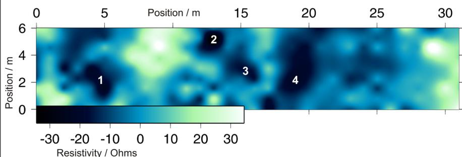
Figure 2: Map view of resistivity data obtained from the crime scene. Four low resistivity anomalies are identified (white numbers).
