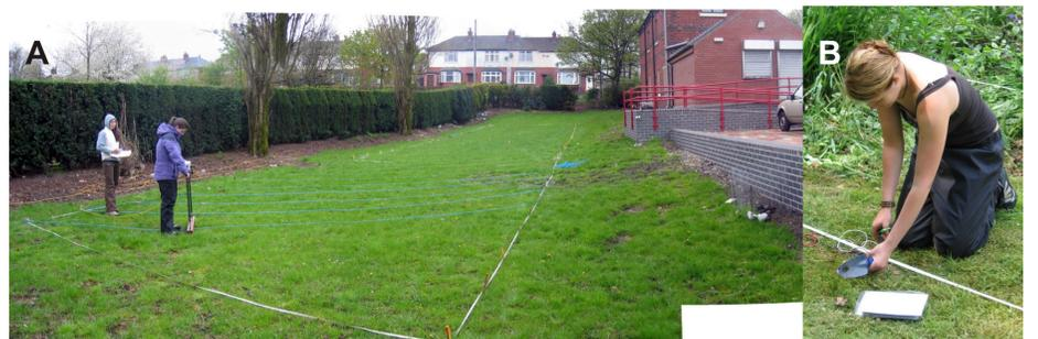
Figure 1: Survey techniques employed in the mock forensic investigation: (a) Lateral Wenner array resistivity and (b) Self Potential (SP). The layout of the crime scene is well illustrated in (a).
