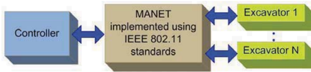
Figure 2 Block diagram of remotely controlled excavator systems (see online version for colours)
