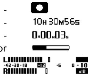
You can PAUSE a recording during record mode by pressing the RECORD button.
